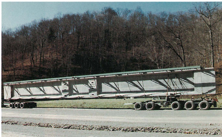
Fig. 13. Transportation of 108 ft (33 m) long bridge beam.
